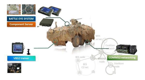
Battle Eye System (BES) is a totally modular application, which separates GUI from GIS and business logic. Task specific modules can be added or removed without the need to recompile the core product. BES relies on Component Server for sensor & weapons integration, on COMMS2 for tactical data communications and on VBS2/3 simulation engine for integrated trainings.
